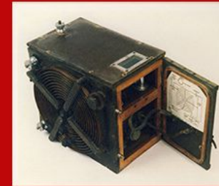
WWI Sterling Set, a morse code spark transmitter, used in aircraft mainly for artillery spotting
